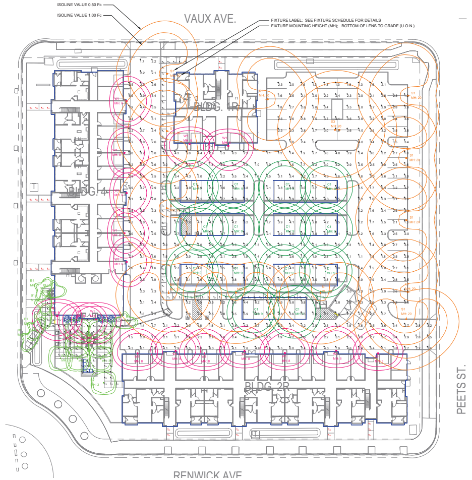
LIGHTING PLAN - PHOTOMETRIC ANALYSIS - LAYOUT VERIFICATION SCALE: 1" = 20'-0" (ALL VALUES SHOWN ARE MAINTAINED HORIZONTAL FOOTCANDLES AT FINISHED GRADE, U.O.N.)
